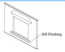
Note: A plastic window pan can be substituted for the sill flashing if the continuous seal of the installation can be maintained. Consult the pan manufacturer for proper installation procedures.
